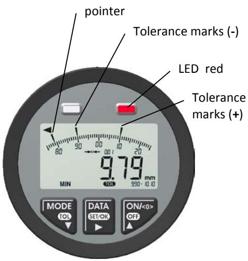
Measuring result **within tolerance**:
